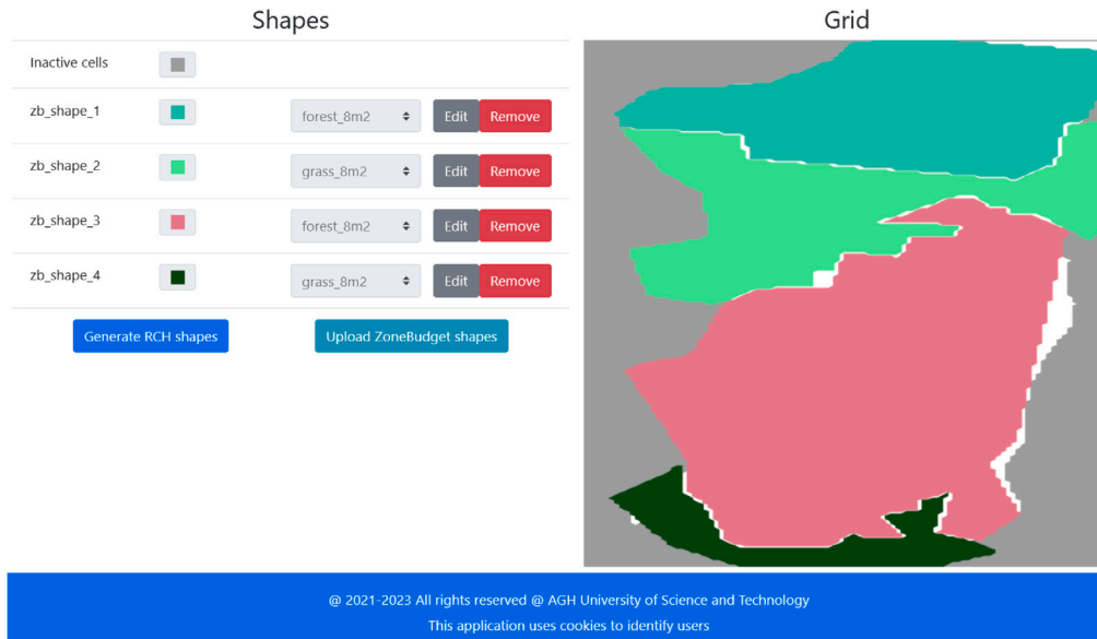
Fig. 3. HMSE interface screenshot showing the assignment of recharge zones.
