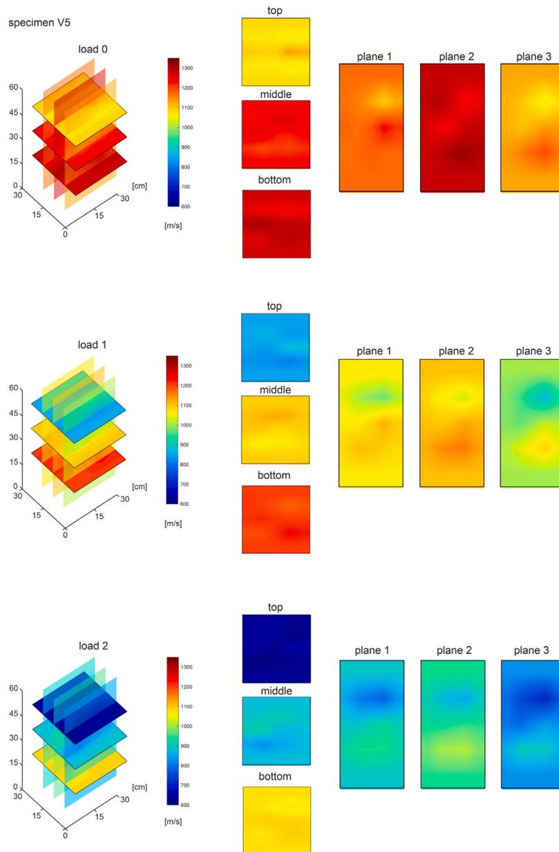
Fig. 22. Results from sonic tomography (specimen V5).
