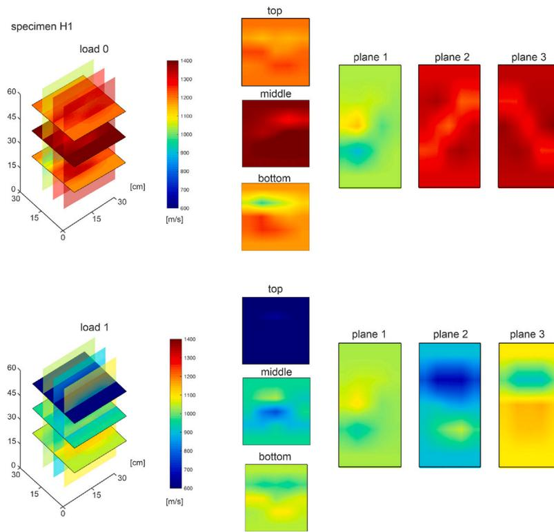
Fig. 12. Results from sonic tomography (specimen H1).
