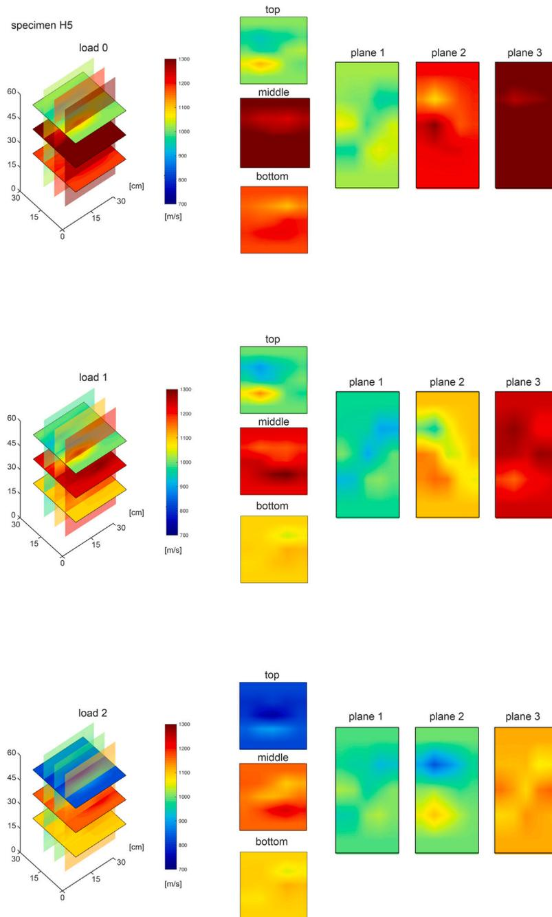
Fig. 16. Results from sonic tomography (specimen H5).
