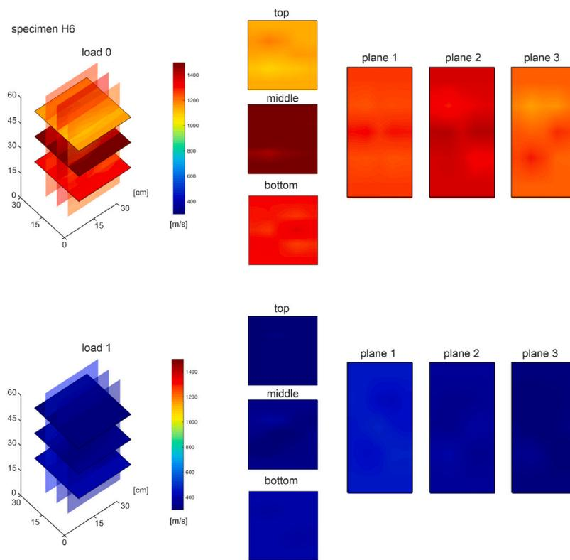
Fig. 17. Results from sonic tomography (specimen H6).
