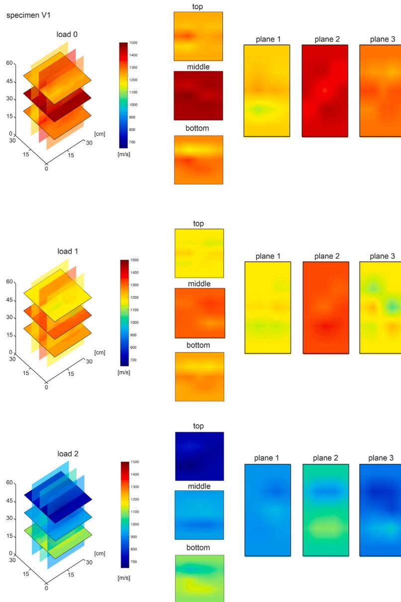
Fig. 18. Results from sonic tomography (specimen V1).
