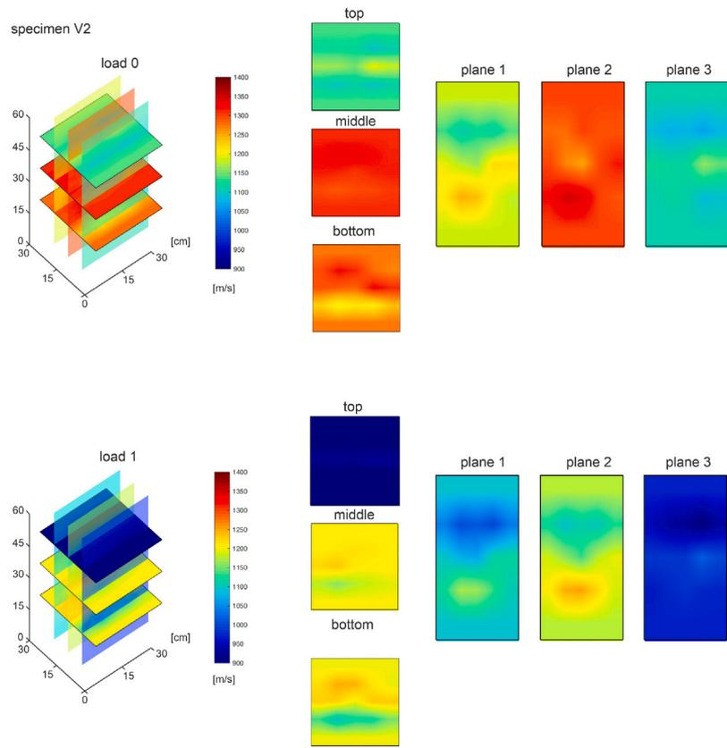
Fig. 19. Results from sonic tomography (specimen V2).
