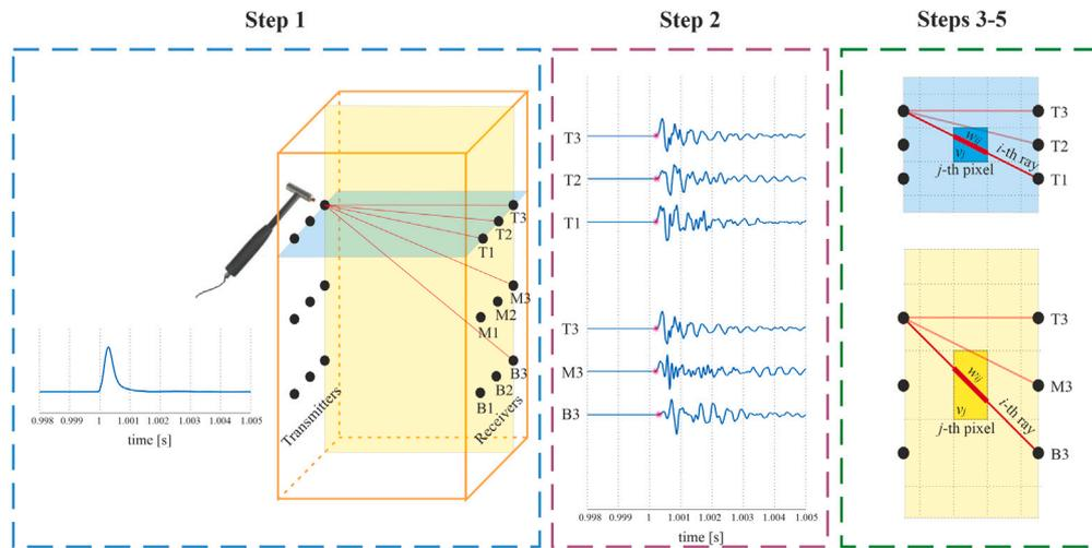
Fig. 5. Illustration of steps 1–5 of tomography algorithm.
