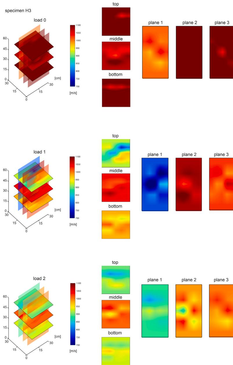
Fig. 14. Results from sonic tomography (specimen H3).
