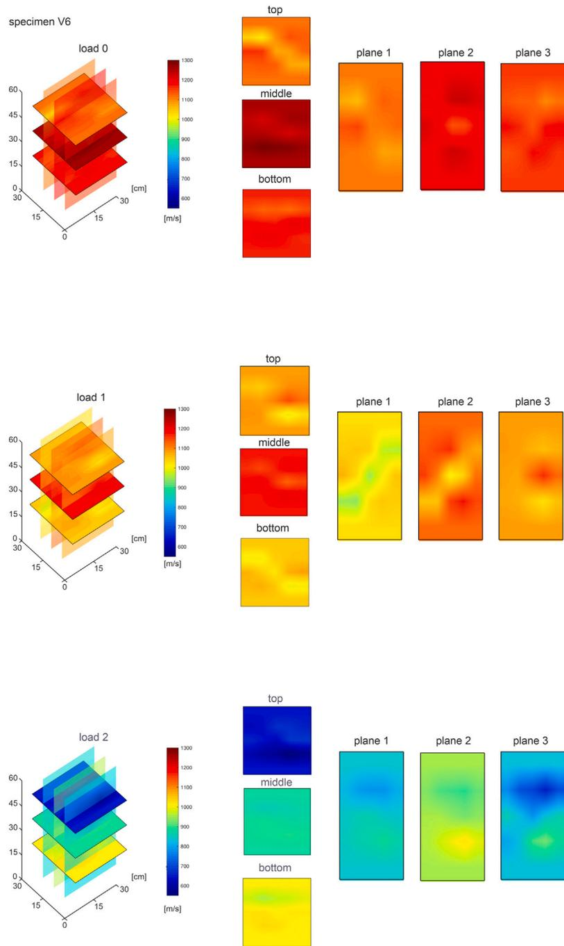
Fig. 23. Results from sonic tomography (specimen V6).
