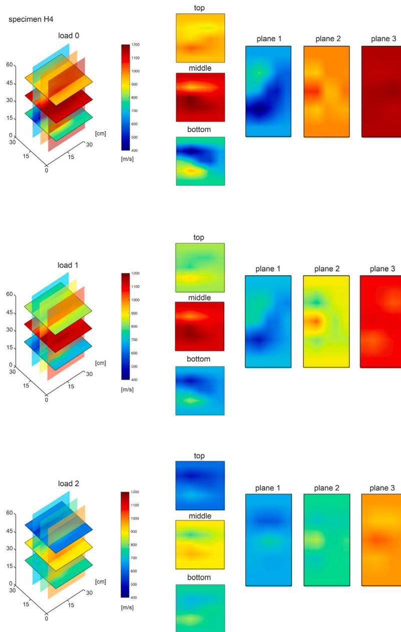
Fig. 15. Results from sonic tomography (specimen H4).
