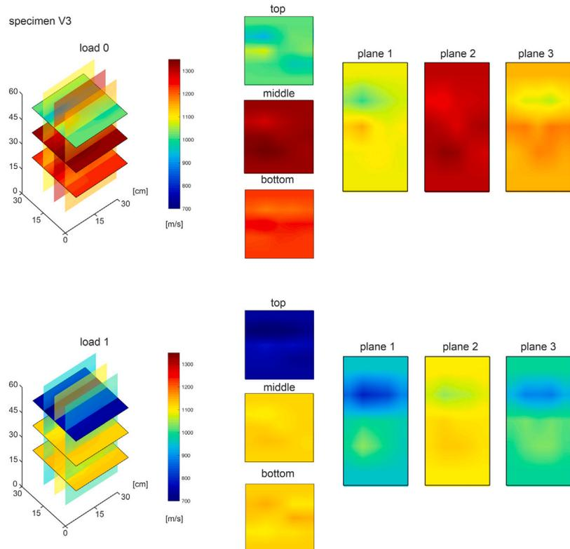
Fig. 20. Results from sonic tomography (specimen V3).
