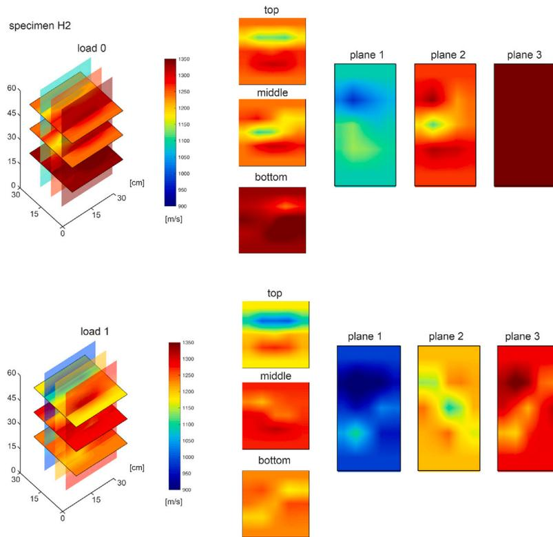
Fig. 13. Results from sonic tomography (specimen H2).
