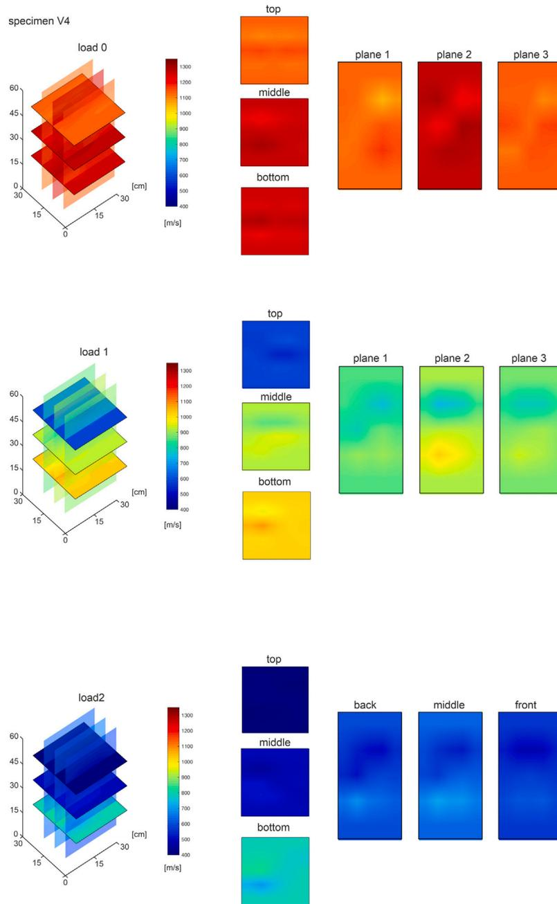
Fig. 21. Results from sonic tomography (specimen V4).
