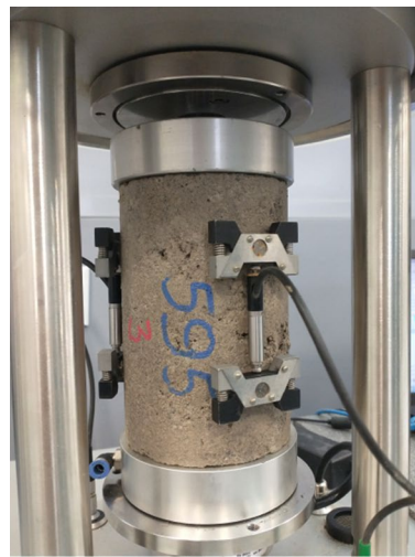
Fig. 2 Simple Performance Tester – test setup: Specimen ready for testing (left) scheme of the test in Simple Performance Tester (right)
