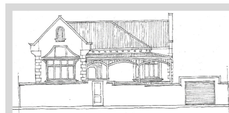
Figure 4-5 - (434 Clark Rd) is one of a number of single residential houses from the Colonial Period that still remain in the overall study area. This house still retains the original detailing of the timber verandah posts, brackets and balustrades. The solid boundary wall and garage door access is a far more recent addition, the typical boundary detail would have been to have a low wall with pillars and cast iron or metal railing infill. The image specifically is included to demonstrate the subsequent compromise of the original streetscape.
