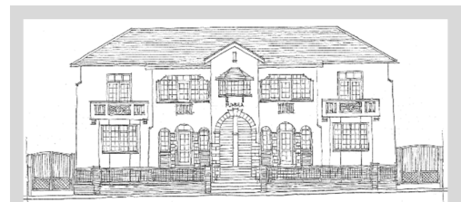
Figure 4-4 - Phumula (64 Hunt Rd) is an exquisitely detailed and maintained Union Period maisonette. Of interest is that there are separate open staircases in the centre of the composition to the two upper floor units.
