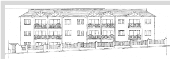
Figure 4-10 - Canberra (65/69 Ferguson Rd) is one of the few Late Century Apartment Buildings in the overall study area, and forms part of one of the detailed street surveys. The use of plaster walls almost exclusively and the hipped gable over balcony volumes is common for the period, as is the double-pitched clay tile roof. The specific concentric square with diagonals timber balustrade module is also rather common for the period. The plaster brick pillar and steel panel infill is original, though the electric fencing topping and stingray spikes is a subsequent addition.
