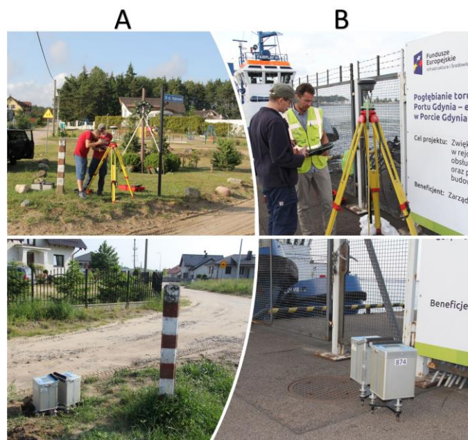
Fig. 1. Gravimeters and GNSS receivers at points of the measurement span: A – POLREF-GORA DONAS, B – Gdynia mareograph.
