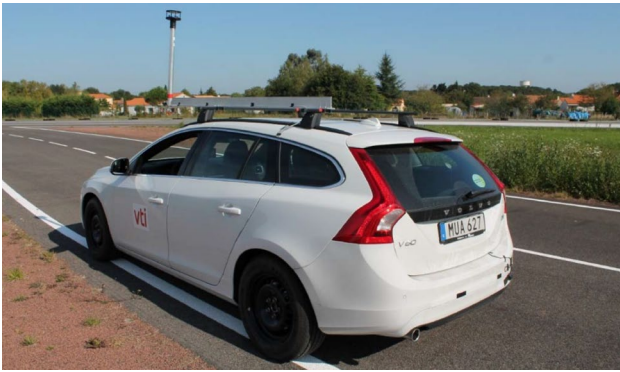
Fig. 1 Test car equipped for coastdown rolling resistance measurements (Anfosso-Ledee et al., 2016)
