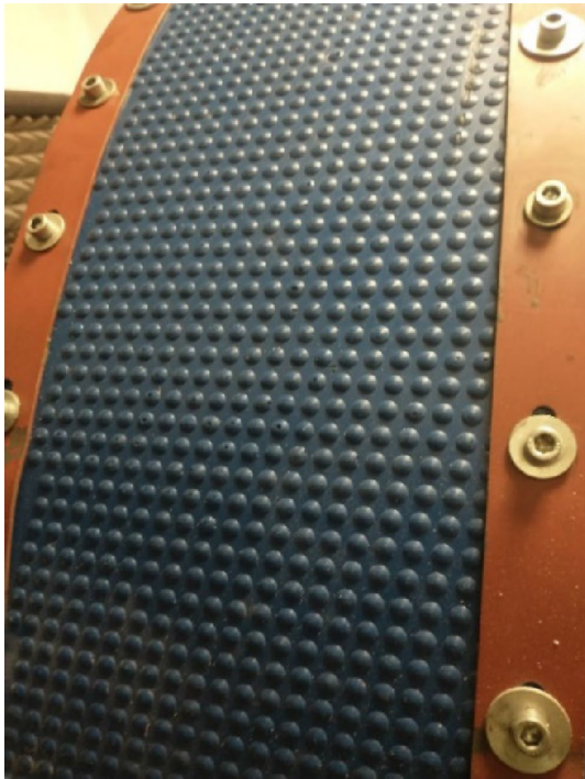
Fig. 14 Example of geometric pattern that may be used for standardized replica road surface for rolling resistance measurements
