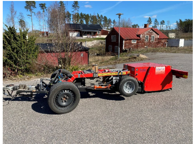
Fig. 2 Test trailer R 2 Mk.3 built by Gdańsk University of Technology
