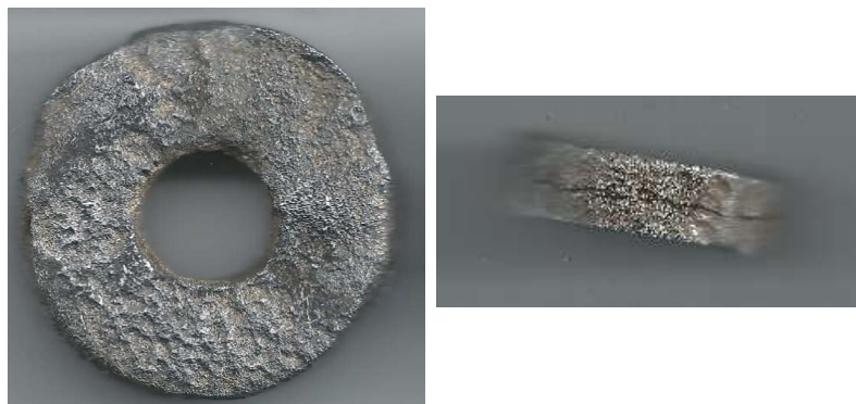
Figure 20. Coupon after 420 days of exposure to aqueous environment saturated with H_2S .
