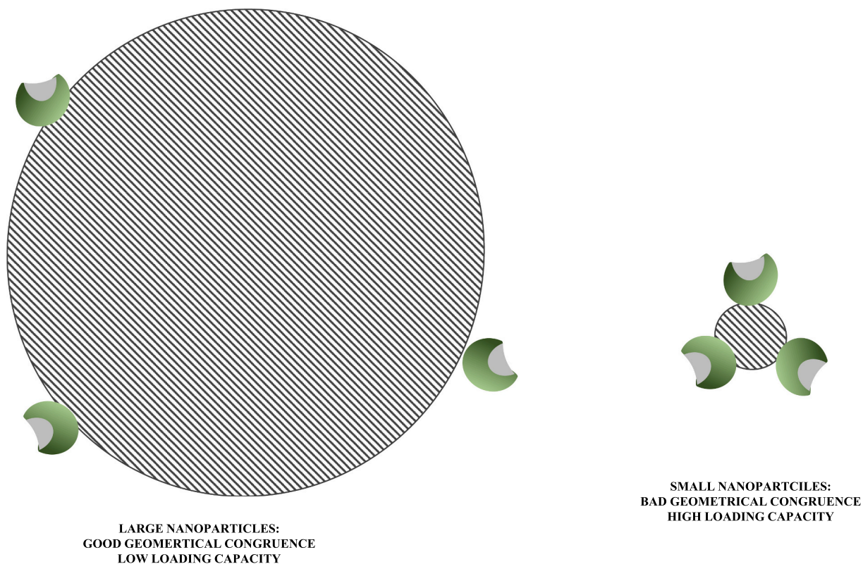
Fig. 20. Enzyme-nanoparticles geometrical congruence dependence on the diameter of the nanoparticle: the smaller the nanoparticle, the smaller the percentage of enzyme surface that can interact with the support.
