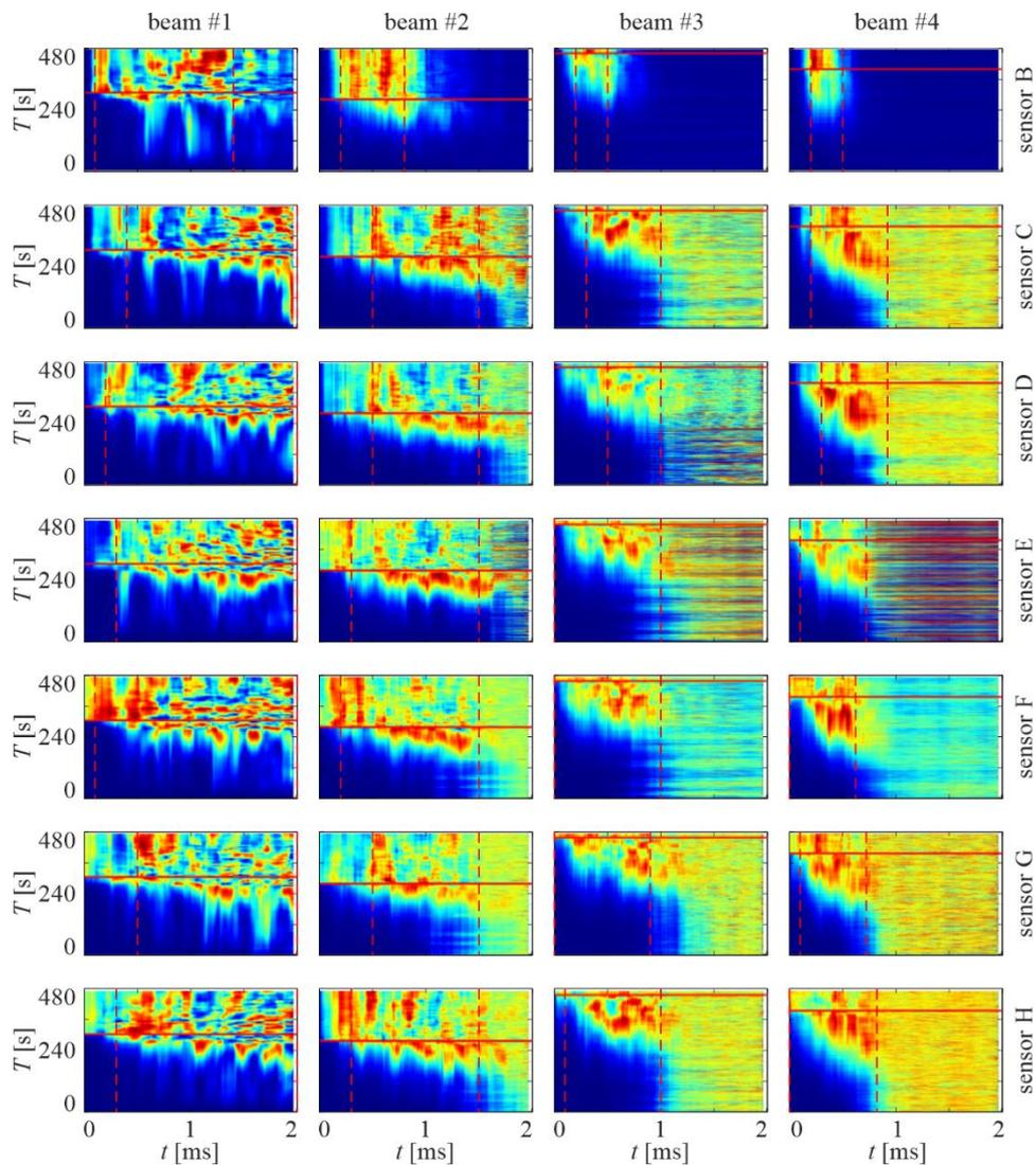
**Figure 4.** Detection of time range of coda waves for beams #1 - #4 and all sensors.
