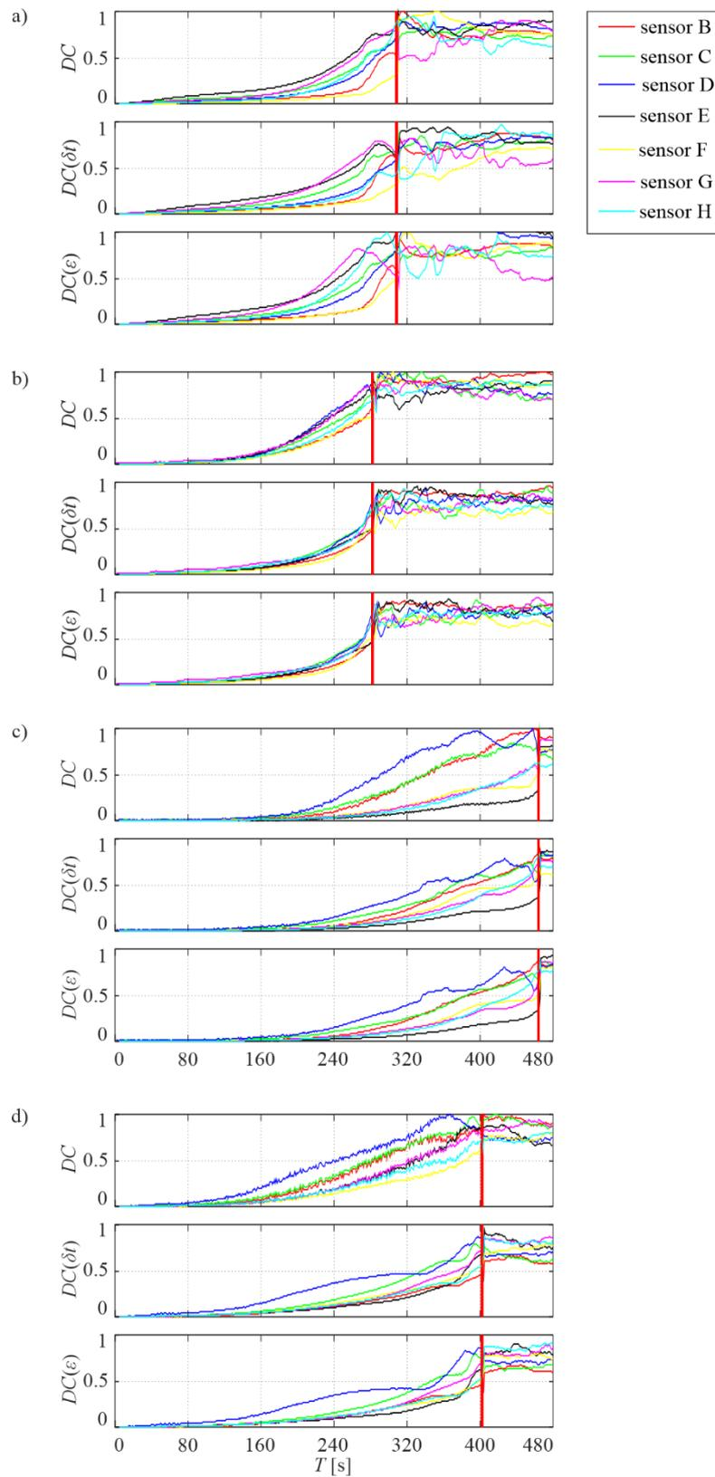
Figure 5. DC for all beams a) beam #1, b) beam #2, c) beam #3, d) beam #4.
