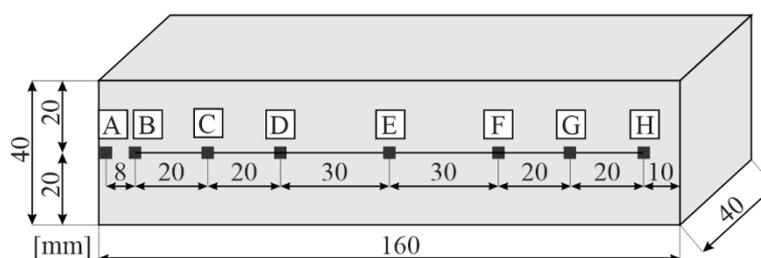
Figure 1. An object of research - specimen geometry.
