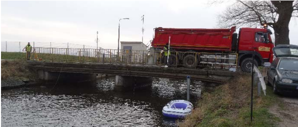
Figure 4. Test load settings: top - inducing a minimum bending moment over the intermediate support, bottom - inducing a maximum span bending moment
