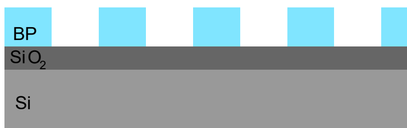
Fig. 4.15 Model used in the analysis of the ellipsometry data.
