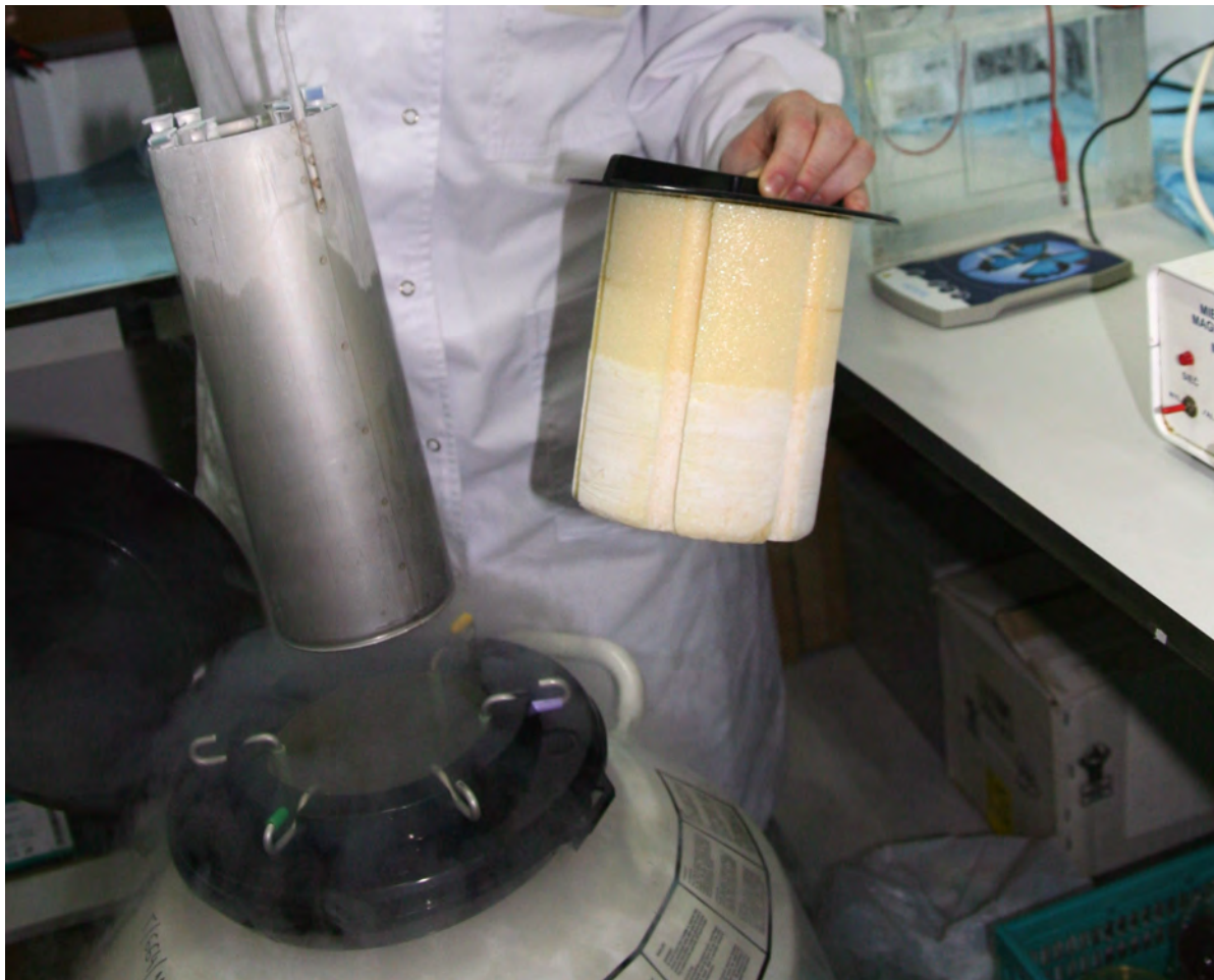
Photograph 4.1.1 Samples during the freezing procedure (under some conditions, microorganisms can survive for a long time); photographed by the Author, 2014
