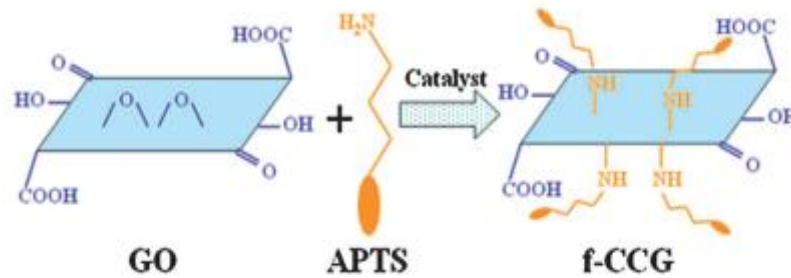
Fig.7 - Illustration of the reaction between GO and 3-amino- propyltriethoxysilane (APTS)[66]
