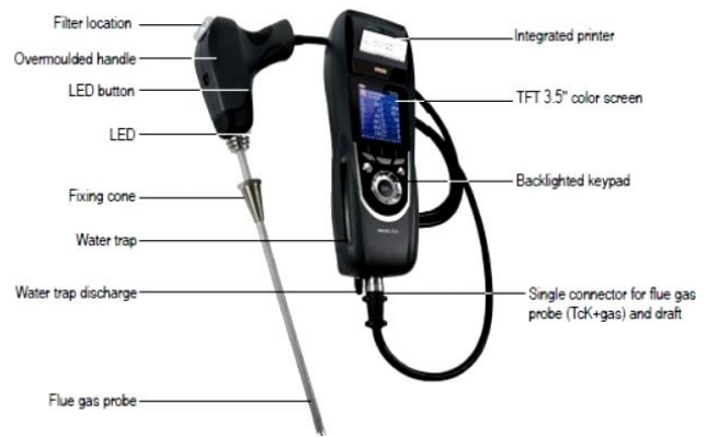
Fig. 3. View of the KIGAZ 300PRO flue gas analyzer used in laboratory tests
