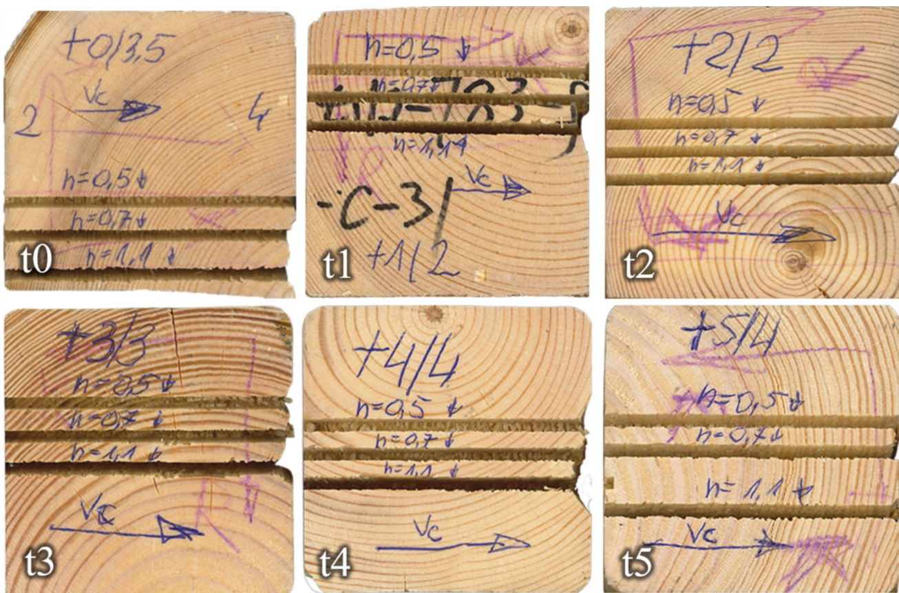
Fig. 1 Cross sections of the clear wood. Three grooves were cut on each of the six cross sections. Cutting direction was left to right, as shown in the picture. The markings on the cross sections are only for
