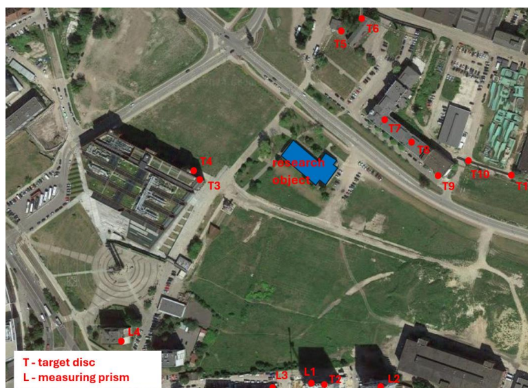
Fig. 10. Sketch of the location of horizontal network reference points
