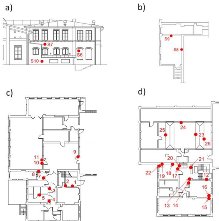
Fig. 11. Location of crackmeters: a) eastern elevation, b) boiler room, c) ground floor, d) first floor
