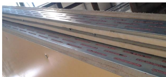
Figure 5. Modified composite sandwich panels: detail of edge reinforcement with perforated steel profiles
