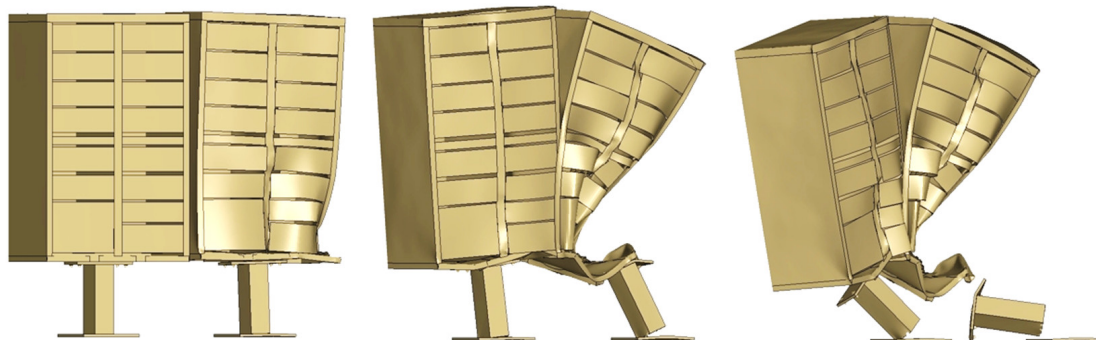
Figure 17. Sequential deformation of the dual-unit Type IV CM impacted by Toyota Yaris at 25° and at the nearest corner on a flat road. Time steps shown are 20, 80, and 120 ms.
