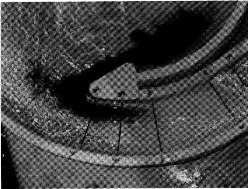
Fig. 9. Water flow between cross-sections v1-v1 and x-x
