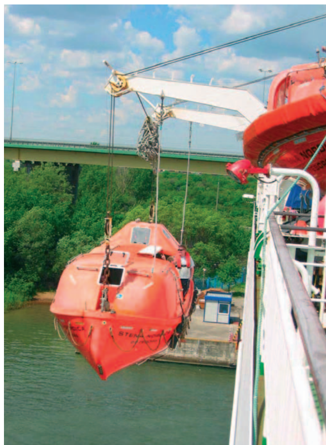
Fig. 1. View of the lifeboat and the luffing jib - traveling davit during defection test .
