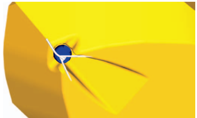
Fig. 3. Isometric view from below. The propulsion unit with the screw propeller of 400 mm diameter .
