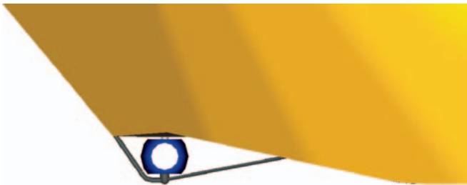
Fig. 5. Side view of the hull. The propulsion unit with the screw propeller of 300 mm diameter.
