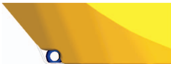
Fig. 2. Side view of the hull. The propulsion unit with the screw propeller of 400 mm diameter .
