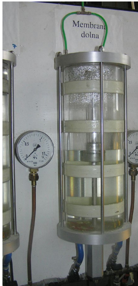
Figure 2. Air-water column with level monitoring with micropulse transducers
