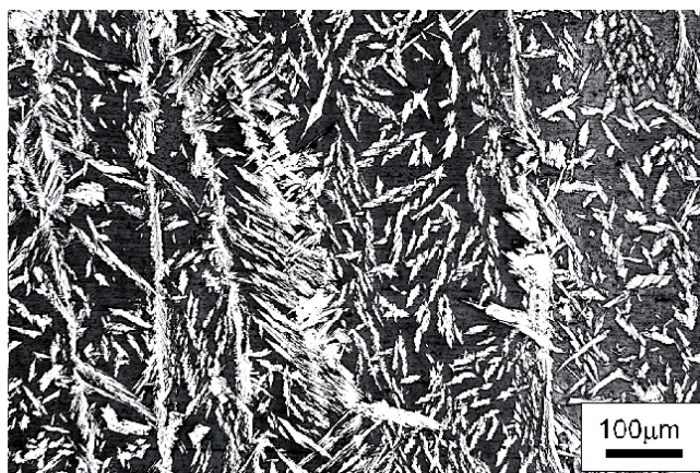
Fig. 2. Microstructure of the welded metal. Y joint, centerline
