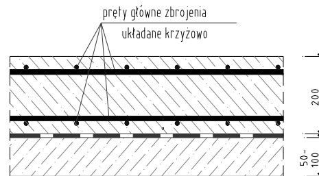
Fig. 1. The floor on the ground (layer arrangement)
