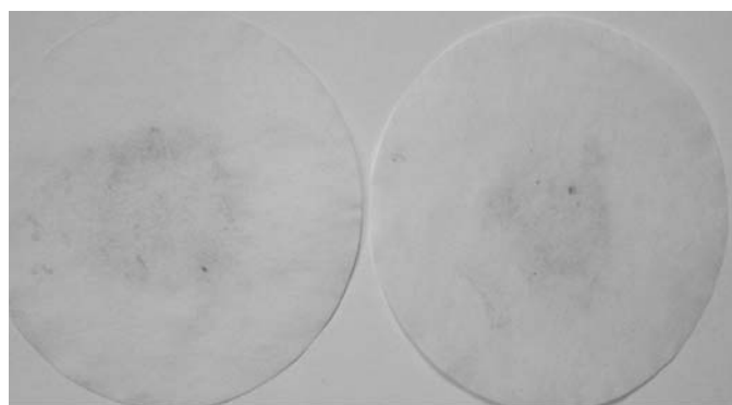
2%, pH 9, corrosion degree: 1
