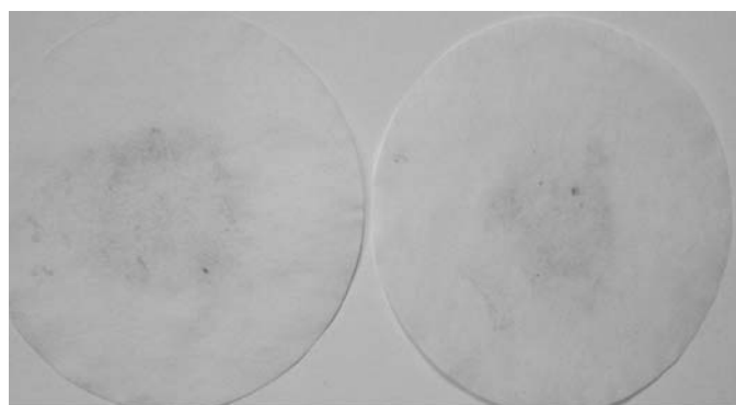
2%, pH 9, corrosion degree: 1
