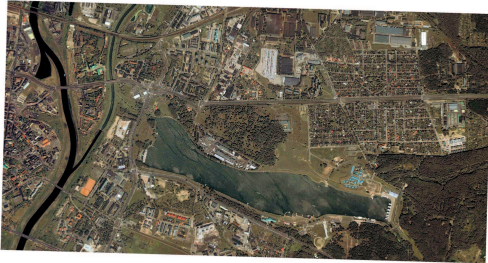
Figure 2. An orthophotomap: scale 1:5000, PUWG 1992 [2]
