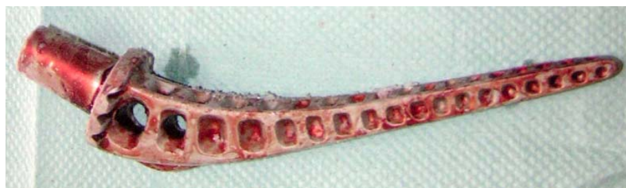
Pic.4. The degraded implants from the first patient
