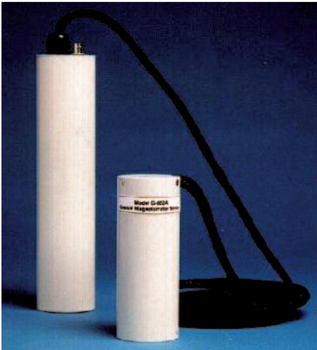
Fig. 10. The optically pumped magnetometer G-822A of Geometrics Company [13]
