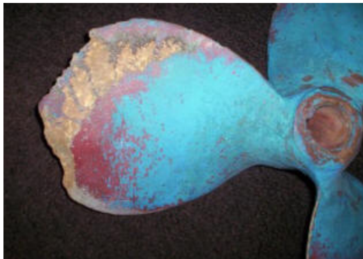
Fig. 1. Cavitation erosion damage of the ship propeller [4]
