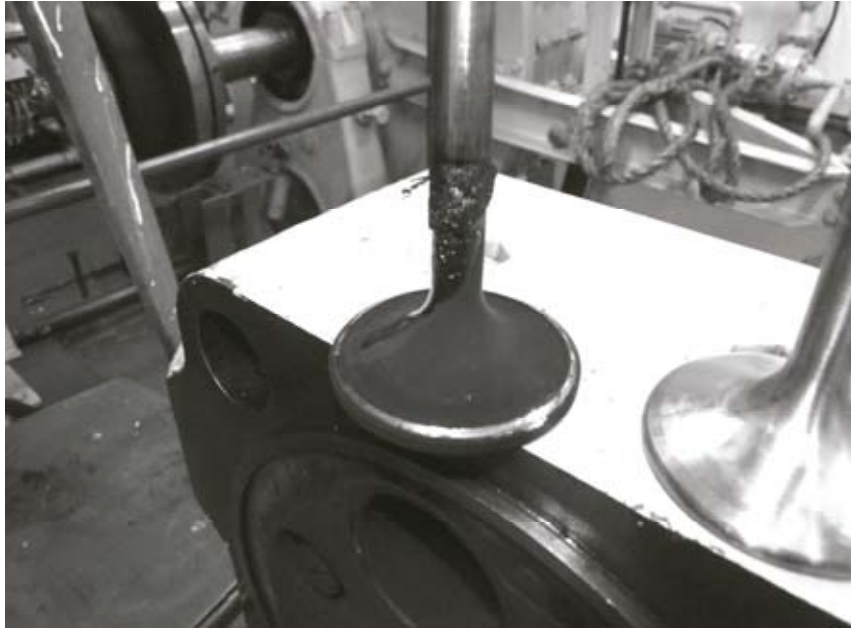
Fig. 3. The valve heads: after service (on left) and new one (on right)
