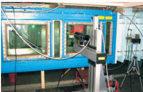
Fig. 3. The laser Doppler anemometer (LDA) ready for measurements of the velocity field around the vortex behind the hydrofoil
