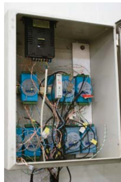
Fig. 11. System of transmitting and recording the data collected from sensors [19]
