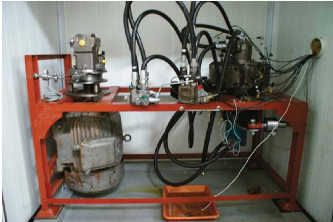
Fig. 10. Laboratory stand for testing hydraulic component [12-17] and system placed in the low temperature chamber
