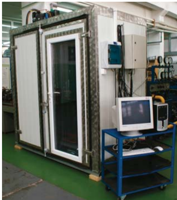
Fig. 9. Low-temperature chamber and measuring system installed in the laboratory of the Chair of Hydraulics and Pneumatics
