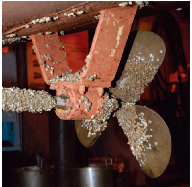
Fig. 2. Cantilever open bearing of yacht's propeller shaft
