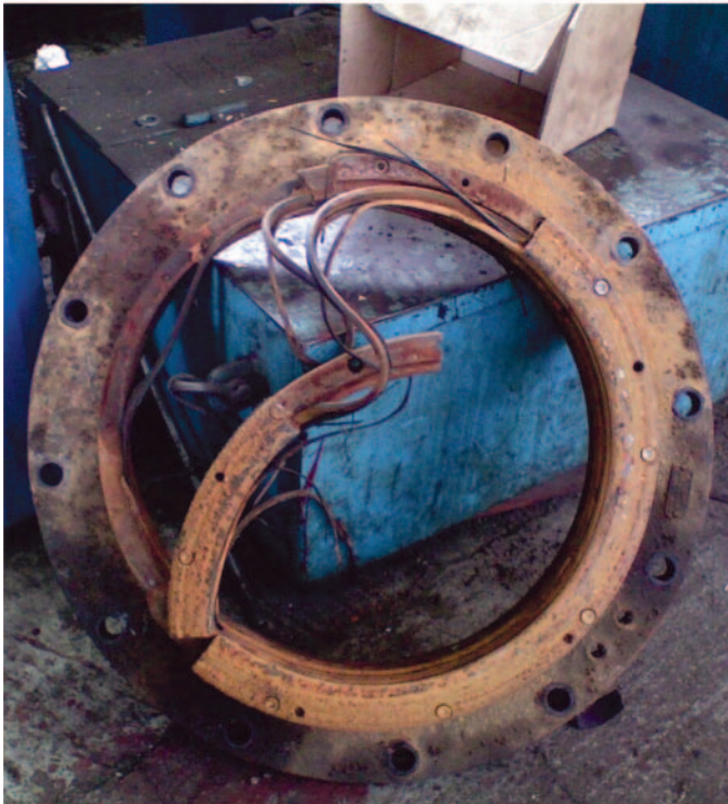
Fig. 1. Completely damaged oil-lubricated slide bearing and sealing of ship propeller shaft
