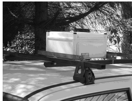
FIG. 1. ARPOL unit mounted on the roof of a car.
