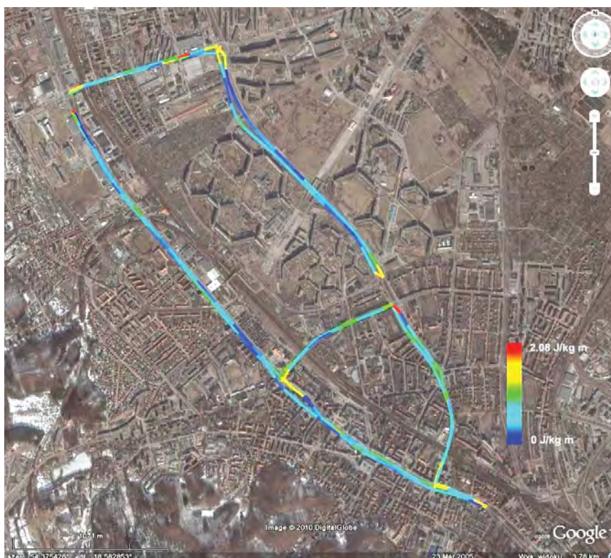
Fig. 2. Map of operating conditions - the specific energy consumption ( \bar{\Phi} )
