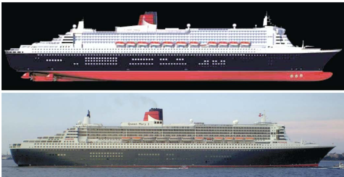
Fig. 1. The ship Queen Mary 2 with visible life boats placed on ship's side [7, 8]
