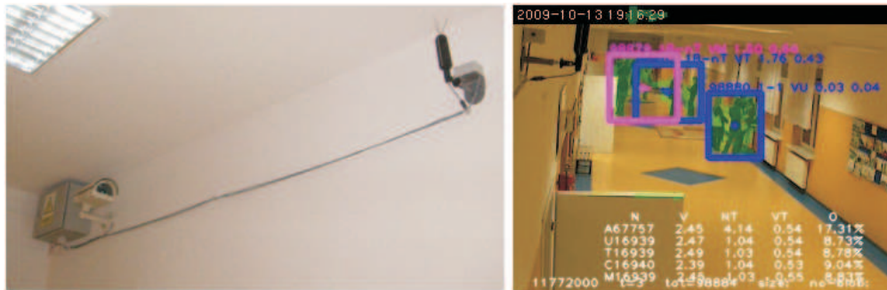
Fig. 4. One of the monitoring stations installed in a school (left), result of the motion analysis for the image acquired by the IP camera (right). Marked rectangles follow discovered “objects” in motion.
