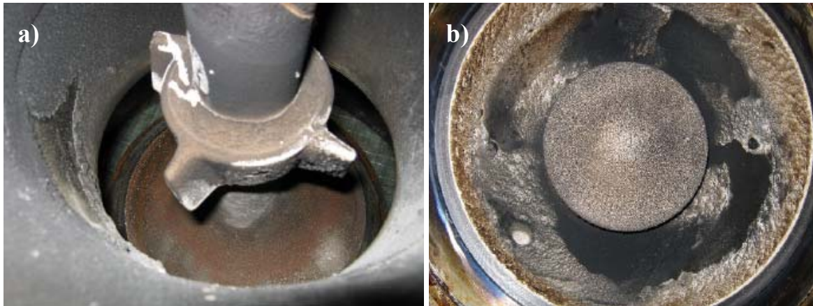
Fig. 3. Exhaust outlet of the port-valve timing system of the 7L35MC-S engine a) exhaust valve stem, b) exhaust valve fungus in the low plate of the cylinder head.
