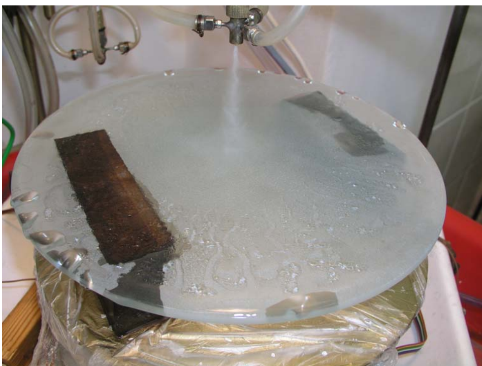
Fig. 16. Phenomenon of re-wetting of liquid layer on a brass surface, following the increase of liquid flow rate from the parameters in Fig. 15 to Re_g=87\ 176 , Re_l=3\ 382 .
