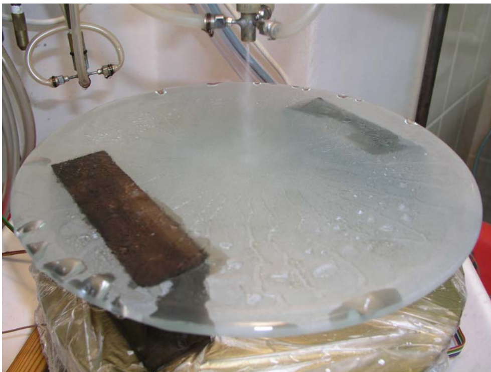
Fig. 15. Phenomenon of breakdown of continuous liquid layer on a brass surface, view after the breakdown, Re_g=88\ 483 , Re_l=1\ 342 .
