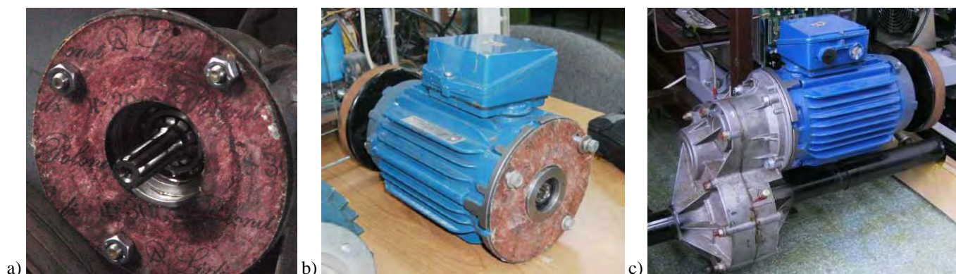
Figure 3. View: a) the input shaft of the differential gear b) motor with driving end shaft (right) and parking brake disc (left), c) AC motor fixed to the vehicle gear
