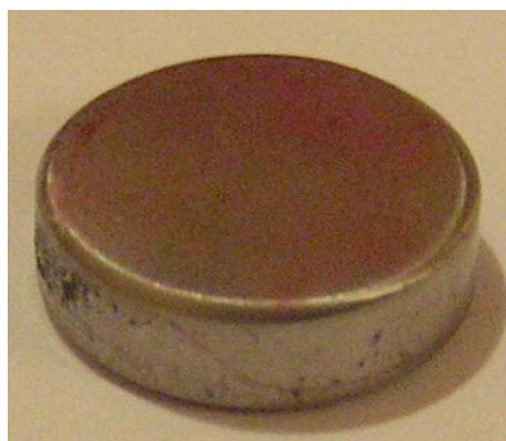
Fig. 5. Appearance of alloy surface after an exposure in Staphylococcus aureus solution
