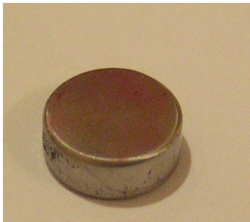
Fig. 4. Samples in the form of discs of the Ti6Al4V alloy
