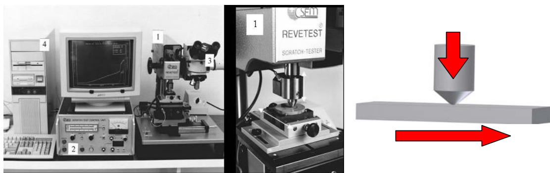
Fig. 5. CSEM REVETEST® Scratch Tester (left) and scratch test contact geometry with the orientation of load and motion vectors marked (right)
