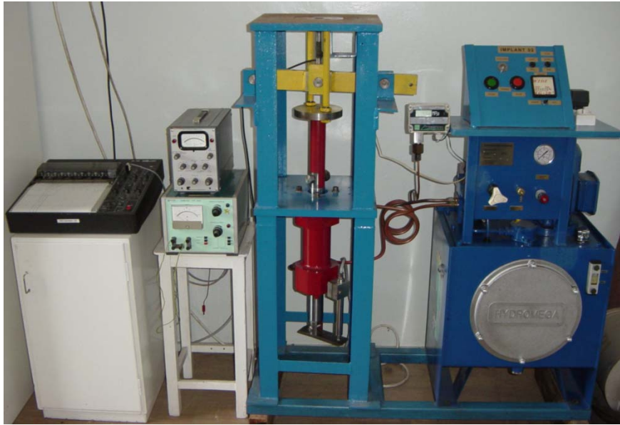
Fig.1. Photograph of IMPLANT 02 test machine
