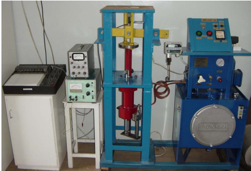
Fig.1. Photograph of IMPLANT 02 test machine
