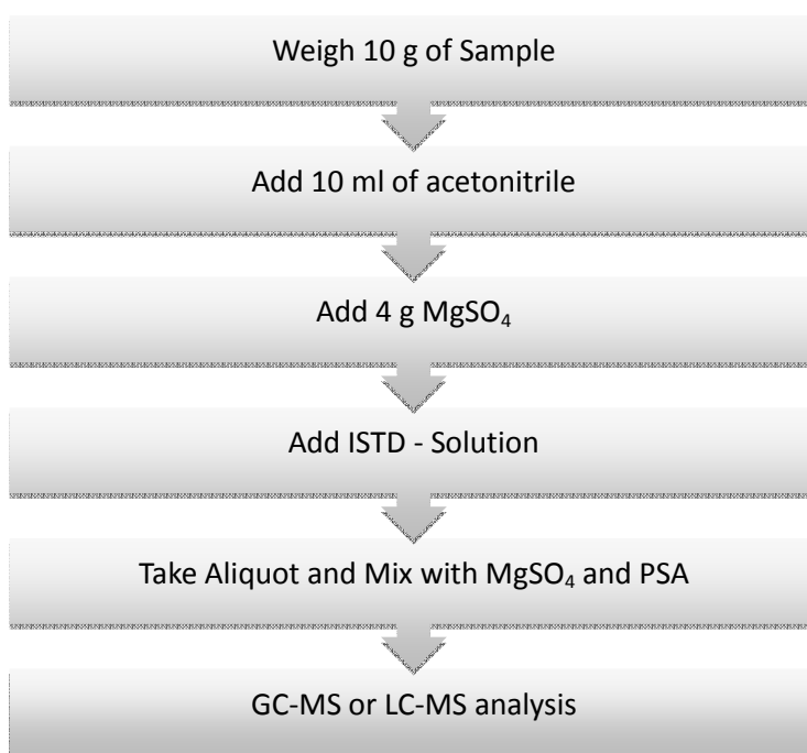
Figure 3. Steps in the QuEChERS procedure of sample preparation for the determination of pesticide residue in fruit and vegetables.
