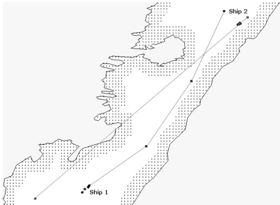
Fig. 2 A trajectory planned for Ship 1 by the typical evolutionary collision-avoidance method
