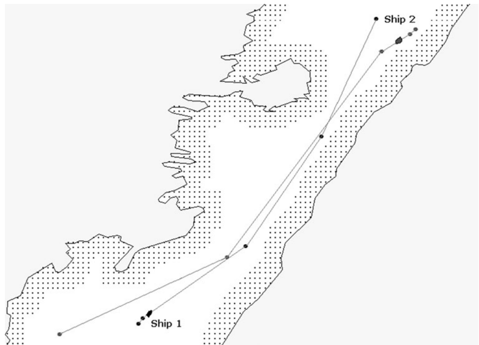
Fig. 4 Potentially dangerous trajectories planned for the two ships by their systems with a single trajectory optimization method applied
