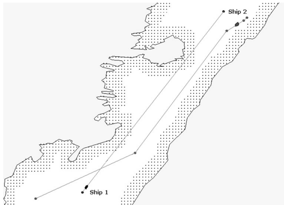
Fig. 3 A trajectory planned for Ship 2 by the typical evolutionary collision-avoidance method
