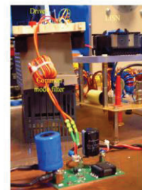
Fig. 1. Automotive DC-DC boost converter fed through the LISN: schematic diagram and experimental prototype view
