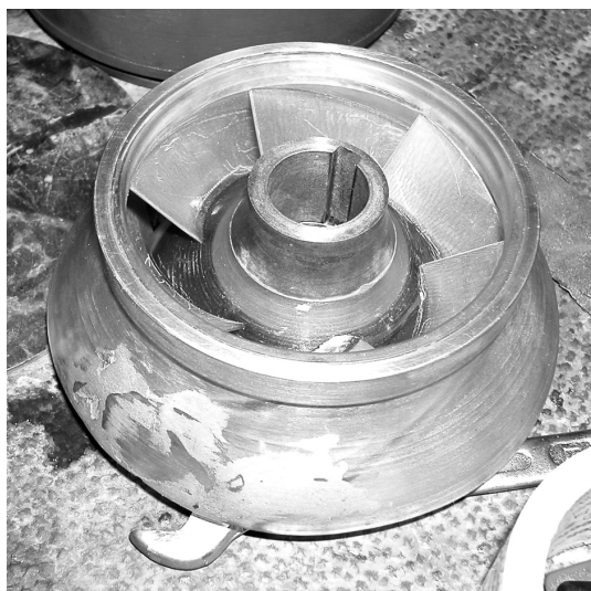
Fig. 4. The pump rotor prototype after testing [10]
