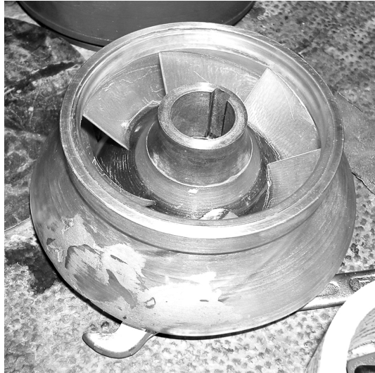
Fig. 4. The pump rotor prototype after testing [10]
