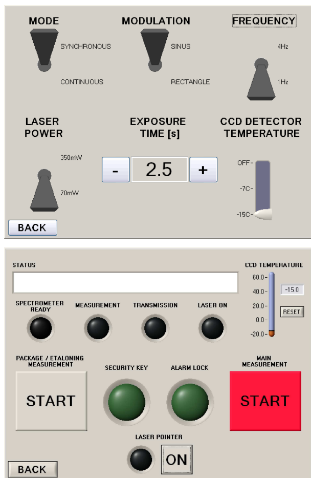
Fig. 2. Front panel of measurement parameters adjustment (top) and the window during the measurement process (bottom)
