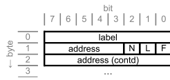
Fig. 3. Binary layout of data fields in a single transition. fsa package compiled with N and L options. N, F and L are bit flags, address field’s length is as large, as the largest state offset in the automaton (but constant for every transition).
