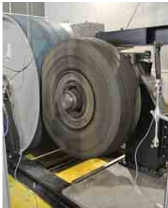
Fig. 3. Roadwheel facility for determination of tyre rolling resistance
